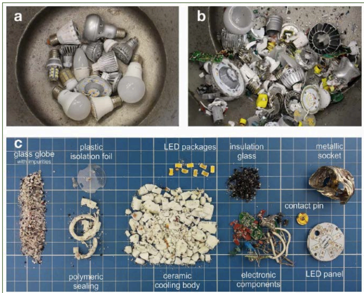
Illustration of the electrohydraulic fragmentation (EHF) method: (a) shows waste lamps before EHF, (b) shows the waste lamps in (a) after EHF, and (c) shows fractions obtained after EHF of one retrofit LED lamp and subsequent manual sorting. 1,7 Photo credit: ©Fraunhofer Project-Group IWKS
